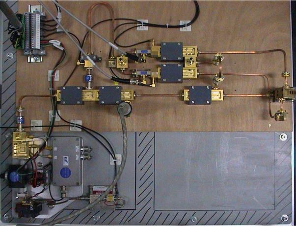
Fig. 2: Photo of the radar front end
