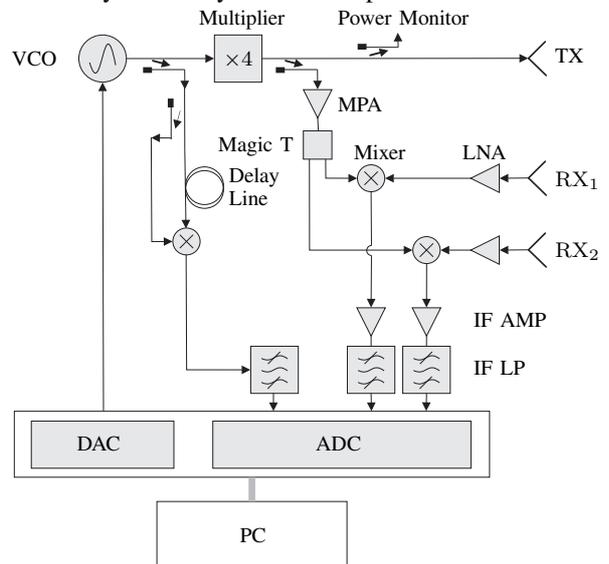
Fig. 1: Schematic of the homodyne MMW FMCW Radar: 1 TX channel and two RX channels
