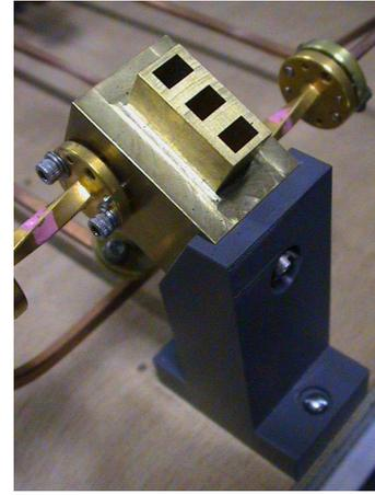
Fig. 3: Milled horn antenna block consisting of three antennas: 1 TX, 2 RX
