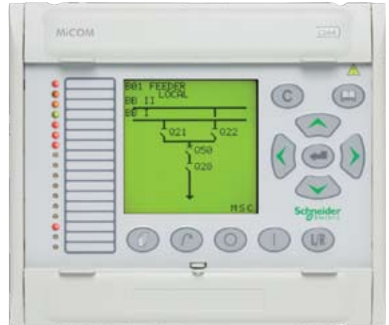
MiCOM C264-P direct operator interface with an optional local HMI
