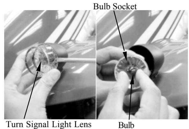
Install the bulb, aligning the bulb socket groove with the bulb tab.
