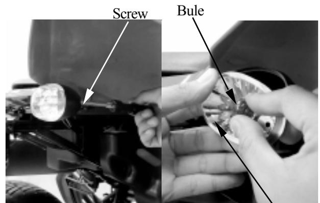
Install the bulb, aligning the bulb socket groove with the bulb tab.
