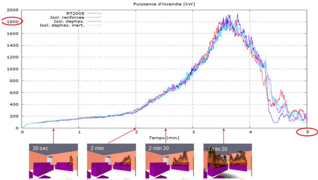
These curves show that in less than 4 min the fire becomes ventilation controlled. If 3 min 40 sec are necessary for the fire to reach his peak (roughly 1800 kW) due to oxygen depletion that power falls to 200 kW in 1min 20s. Walls composition influence over the fire power is not significant for this time scale. At most the difference between one wall and another is 100 kW, which is insignificant.
