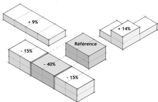
Comparison of heat loss due to the envelope of a building (for 96 m<sup>2</sup> housing). For the same surface, limiting faces in contact with the outside could result in non negligible savings. Semi detached two floor structure should become a model for standard construction.
