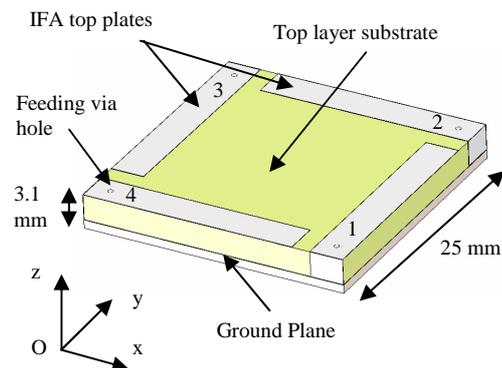
Figure 1: Structure of the four Inverted-F Antennas.
