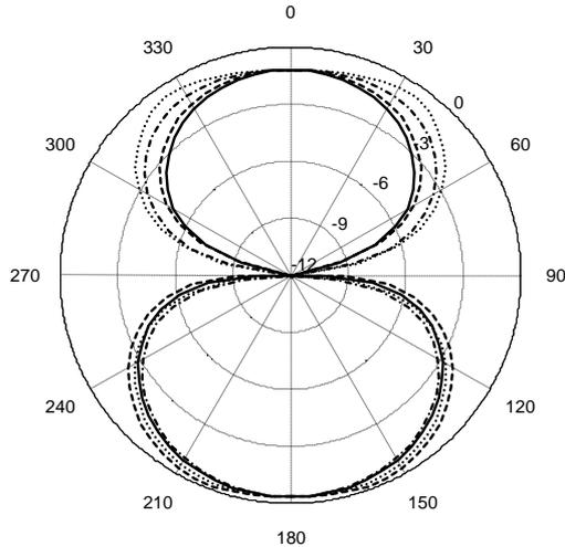
Figure 9: Axial ratio pattern (dB) for different OZ planes at 2.4GHz (0dB = circular polarization)
