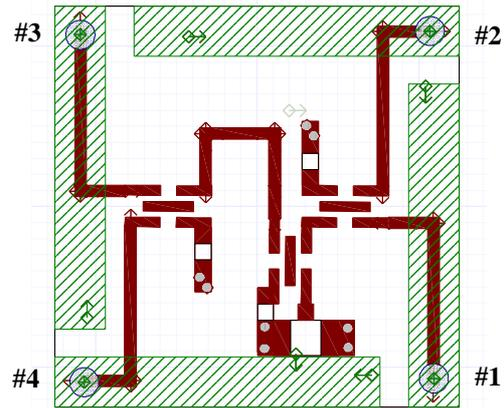
Figure 4: Layout of the microstrip network.
