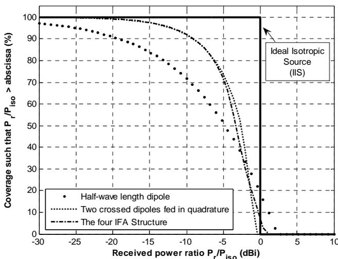
Figure 10 : Isotropic coverage of the four IFAs structure compared to 3 well-known antennas.
