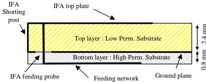
Figure 2 : Dual layer stackup and arrangement of the Inverted-F antenna
