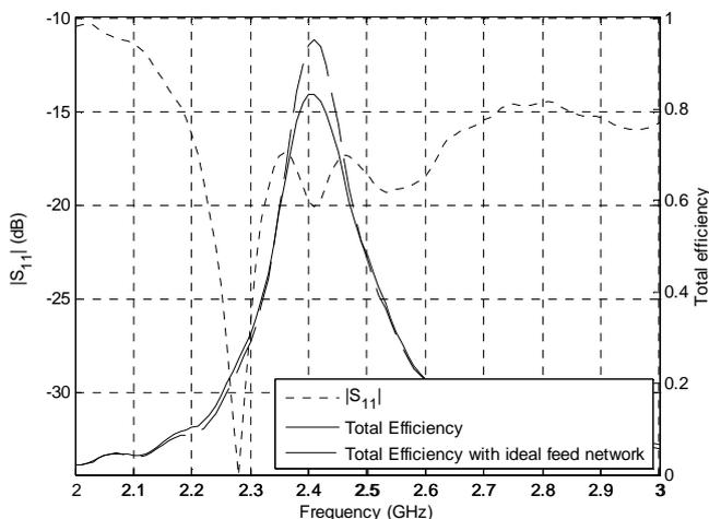
Figure 7: Impedance matching at network input and antenna total efficiency.
