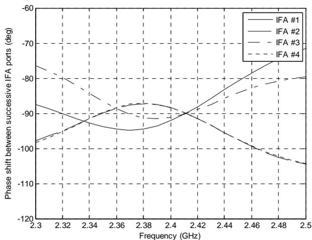
Figure 6: Phase shift between successive IFA ports.
