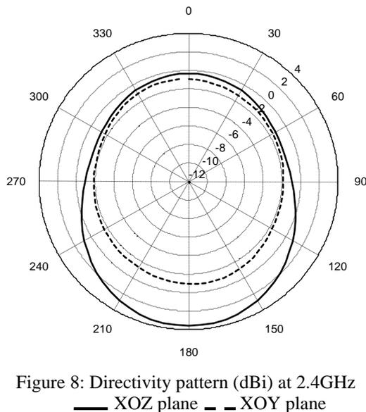
Figure 8: Directivity pattern (dBi) at 2.4GHz
