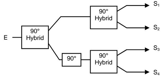
Figure 3: Schematic of the feeding network for equal amplitude and 90° phase shift between successive outputs.
