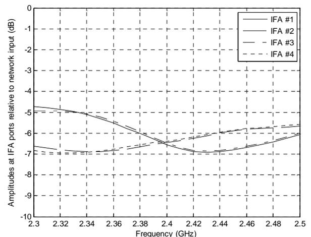
Figure 5: Amplitudes at IFA ports relative to network input.
