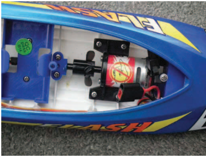
Brushed motor with cooling fan
