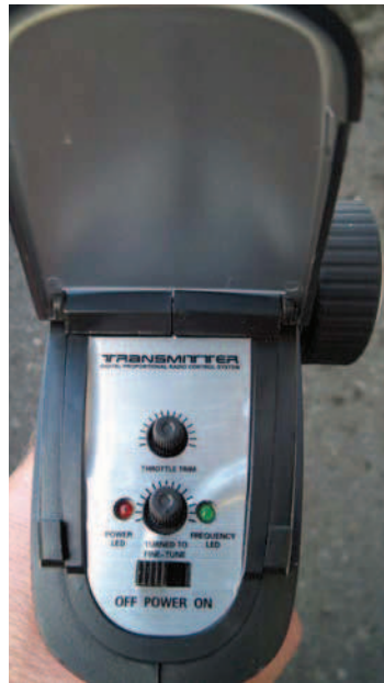
The pistol grip transmitter showing the trim adjustments and function LED's
