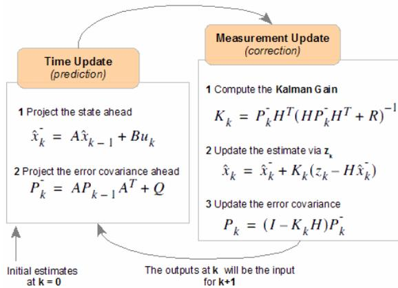
Fig 2. Diagram of the different steps to compute the position within a Kalman filter
