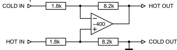
This is a difference amplifier. Gain is not quite 8.2k/1.8k because of the finite gain of the switching output stage. It works out as 4.5 times.
