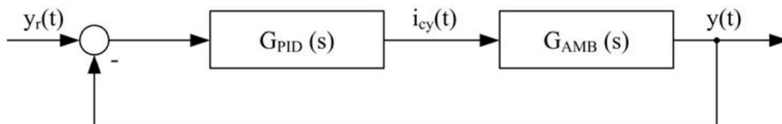
$$G_{CL}(s) = \frac{\frac{K_D k_{iy}}{m} S^2 + \frac{K_p k_{iy}}{m} S + \frac{K_I k_{iy}}{m}}{S^3 + \frac{K_D k_{iy}}{m} S^2 + \frac{K_p k_{iy}}{m} S + \frac{K_I k_{iy}}{m}} \quad (13)$$
