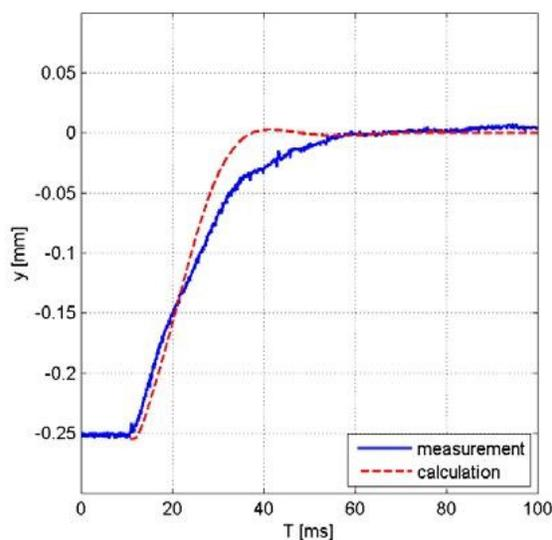
**Fig. 14.** Time response of the AMB shaft displacement in y-axis
