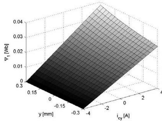
Fig. 9. Flux characteristic  $\Psi_I(i_{cy}, y)$
