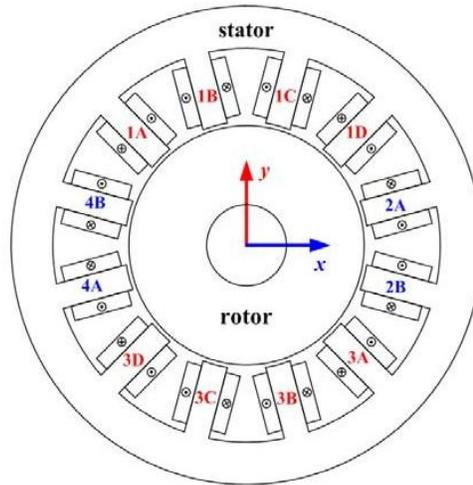
Fig. 1. Front view of the active Magnetic bearing
