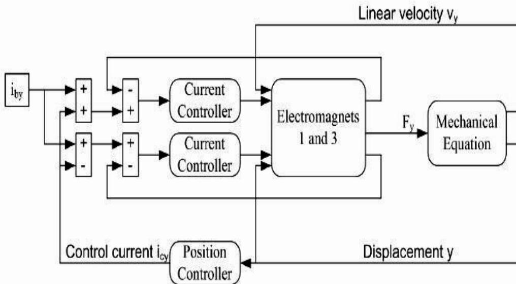
Fig. 3. Block diagram for the analysis of the AMB dynamics in y-axis
