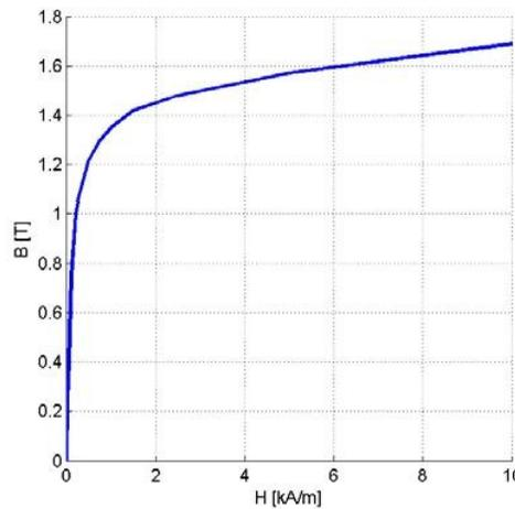
Fig. 2. B-H characteristic for the laminated ferromagnetic material M270-50
