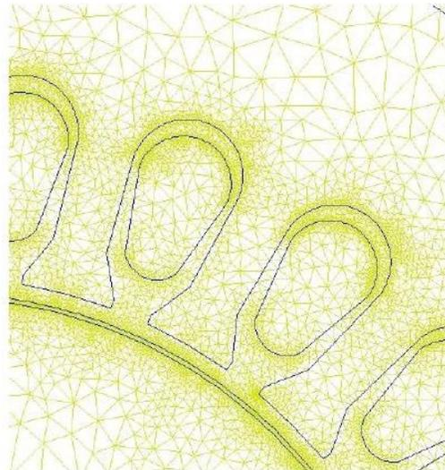
Fig. 6. The finite element mesh in the subregions of stator and rotor
