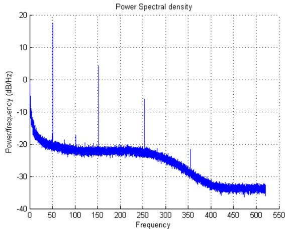
Figure 4: Power spectral density with electrodes set to ground
