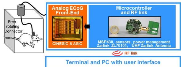
Figure 3: Experimental set-up with ECRINS board and CINESIC8
