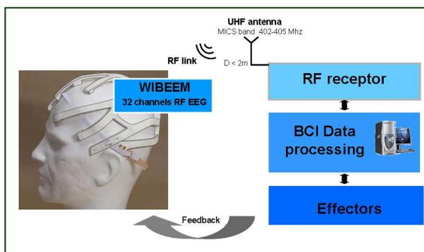
Figure 8: The experimental set-up for WIBEEM
